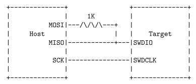
The 1K resistor works well with most MCUs up to 3 MHz. A lower resistance could be used to achieve higher speeds granted that the target SWDIO pin has enough drive strength to pull the signal high while being pulled low by this resistor.
